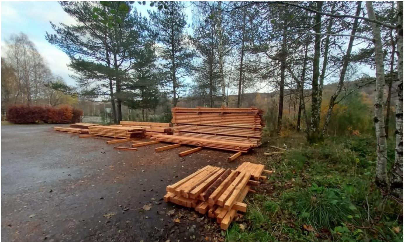
Stacking the timber properly is important, it'll remain here for about 6 months
